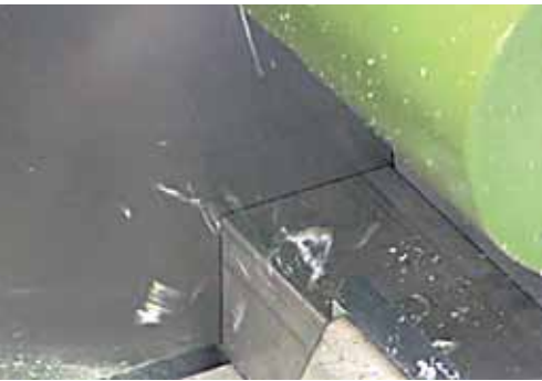
Sawing is an ideal application for MQL.
