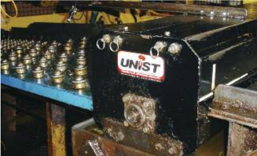
A roller unit sits ready to apply an even, thick film of drawing compound top and bottom at the entry end of a press.
