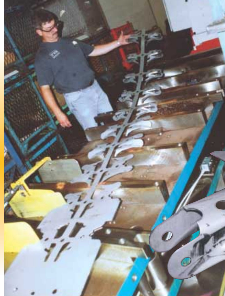
TT&D likes the flexibility offered by its programmable lubrication stations, so that its ability to lubricate dies doesn’t limit the type of job in can run. It won this job—upper-suspension control-arm brackets—in March 2002. Running the 12-station progressive die, lubrication is provided by a roller at the entry end complemented by four nozzles in the die—two at the form station and two more at the cam-pierce station.
