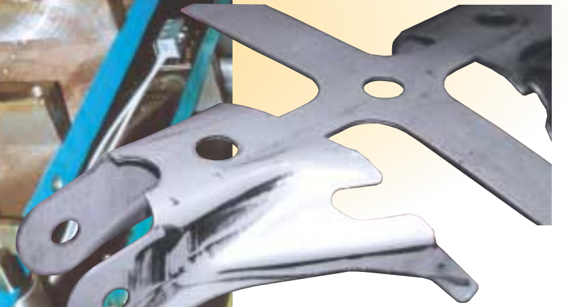
TT&D likes the flexibility offered by its programmable lubrication stations, so that its ability to lubricate dies doesn’t limit the type of job in can run. It won this job—upper-suspension control-arm brackets—in March 2002. Running the 12-station progressive die, lubrication is provided by a roller at the entry end complemented by four nozzles in the die—two at the form station and two more at the cam-pierce station.
