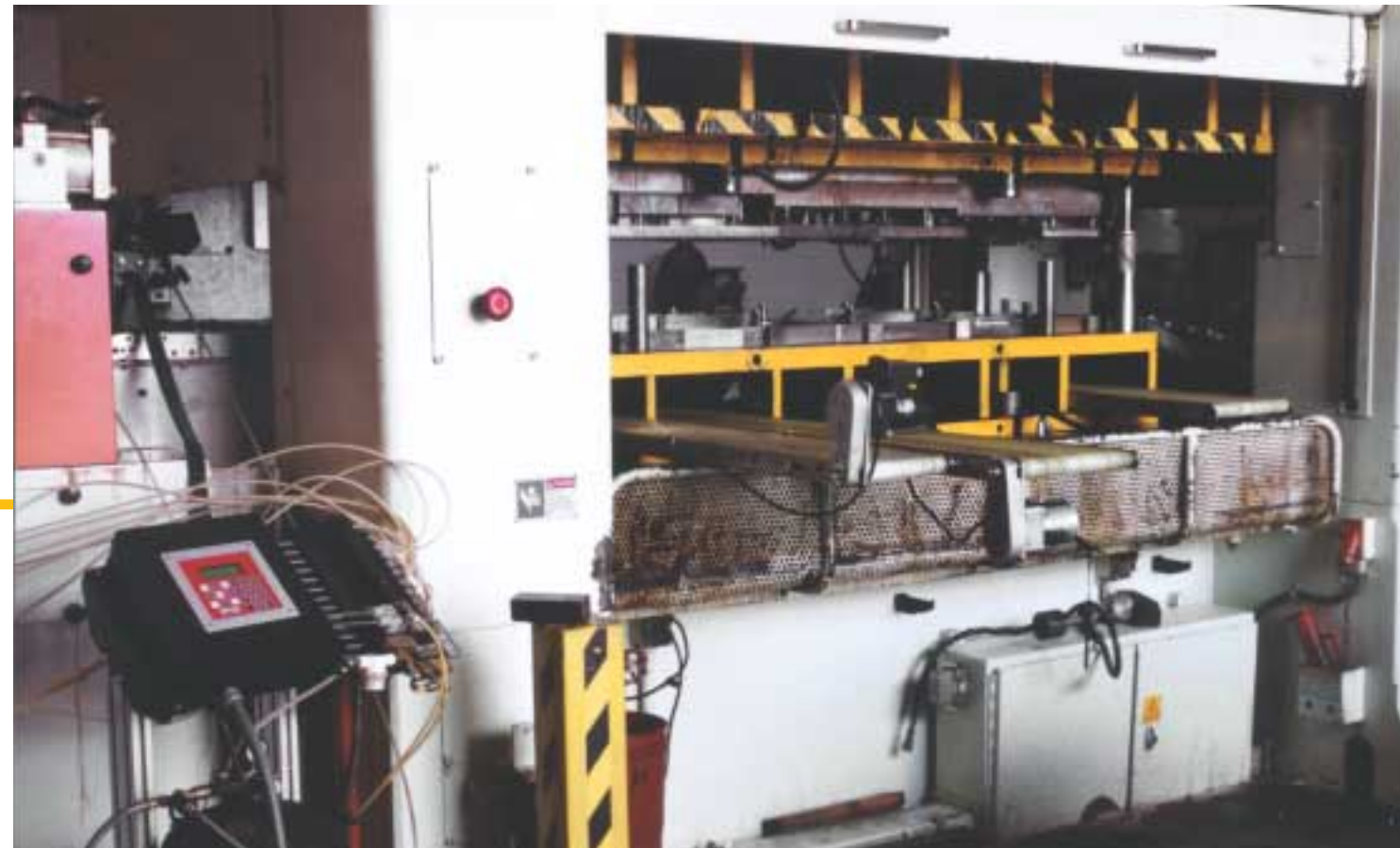
A programmable lubrication station (left) installed on a press at Toledo Tool & Die directs lubricant flow to a roller (top left) and to several nozzles located in the die. Lube procedures can be set, tweaked and optimized, then saved with each die. Menu-driven software eases programming, and an access code protects the setups.
